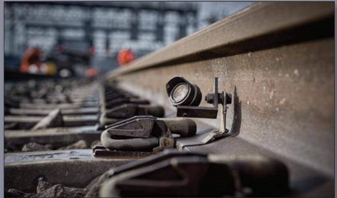
One of more than 600 prisms attached to the track. The Trimble software combined optical measurements with data from tilt sensors.
