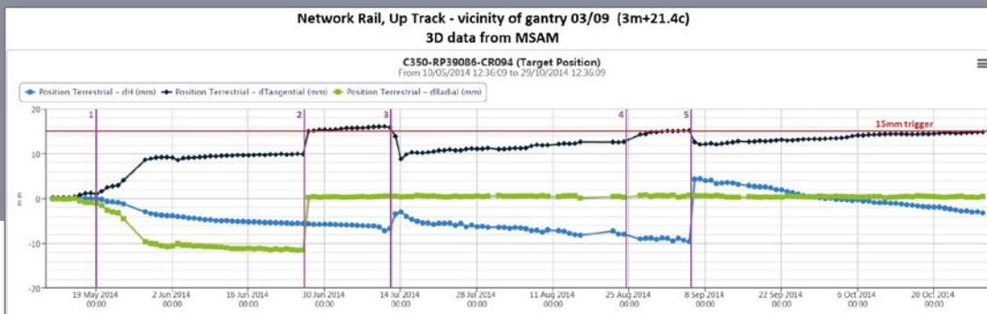
Measurement data for a single prism reveals changes in three dimensions. Each prism was measured on an hourly cycle.
