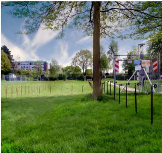
Left: To monitor the “soft” areas of the tunnel corridor, iron rods with prisms were driven into the open fields/parks in dense arrays.
