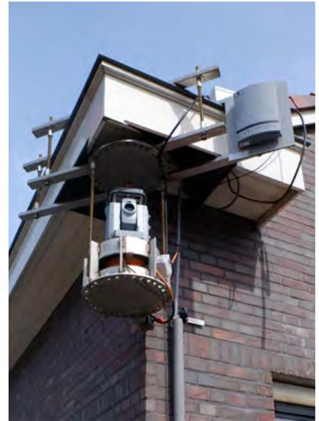
Monitoring robotic total stations were mounted on solid posts in secure enclosures along the route. These self-contained monitoring units have robotic total stations, communications radios/-modems, rain/snow hoods, and sometimes cameras. They operate as a connected network of instruments and common inter-visible monitoring/control points.
